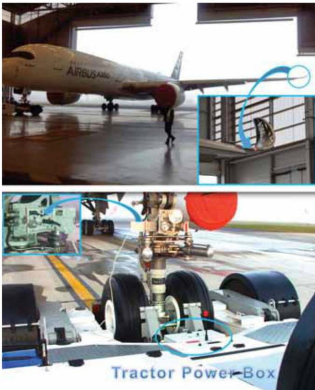
Figure 3: Aircraft navigation lights powered by a towbarless tractor
