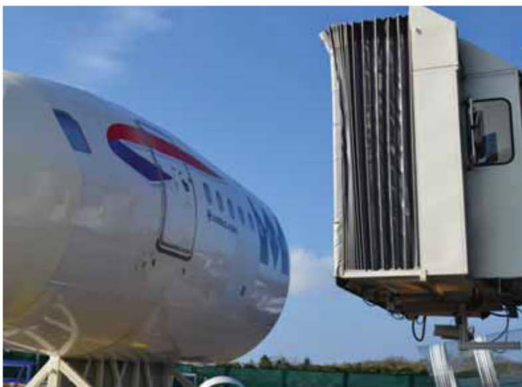
Figure 2: Passenger boarding bridge automated docking tests
