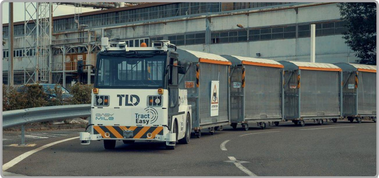
The TractEasy® has been co-developed with the French company EasyMile. Its mission is to move cargo in an autonomous manner, under the supervision of dedicated fleet manager software, from terminal to terminal, or terminal to aircraft.
