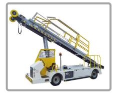
TLD offers 3 NBL models in this product line, diesel NBL (37-44 kW range internal combustion diesel engine) and NBL-E, an Electric version with leadacid or Li 80VDC batteries. Duty cycles considered are identical at 1,000 hours per year, but no idling (45%) on electric version, lifetime 12 years.
