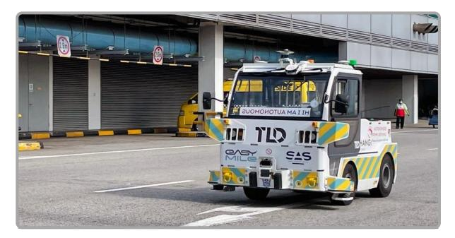
The TractEasy<sup>®</sup> has been co-developed with the French company EasyMile. Its mission is to move cargo in an autonomous manner, under the supervision of dedicated fleet manager software, from terminal to terminal, or terminal to aircraft.
